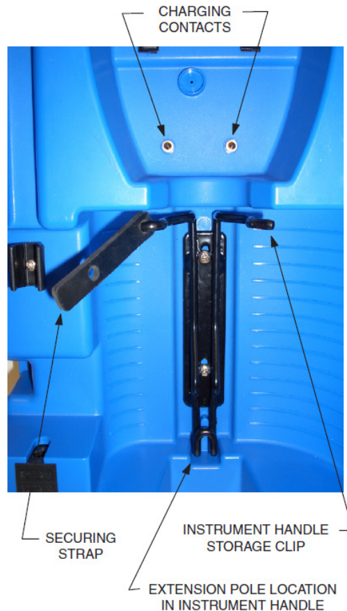
Figure 40: Charging Station - Monitor Location
